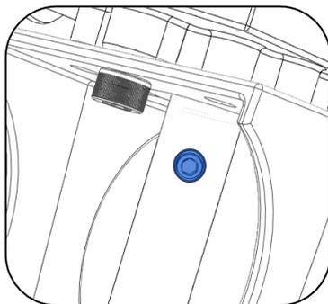
For a backlash-free connection, tighten the optional upper socket set screw on the actuator shaft (if available). If the actuator is to be dismantled, this must also be loosened before.
